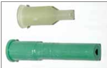
Figure 3 The small white cooling nozzle on the top was used pre-1991; in 1991 Cummins went with a higher volume oil pump and switched to the larger nozzle shown on the bottom. Regardless of the model year of the engine, the use of the larger nozzle with the higher volume oil pumps is recommended.
