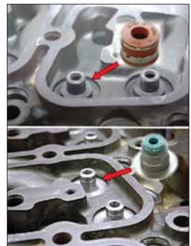
Figure 9 The upper image shows the early design seal with sharp machining edges in spring pocket area. The lower images shows top hat type seal with radius spring pocket area.
