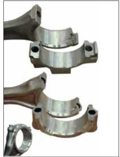
Figure 6 The first and second series rods have “tongue-groove” design rather than the “cracked” parting line of the third design. The third design rod also has mirrored machined bearing tangs and uses two different bearing halves between upper and lower (see inset).
