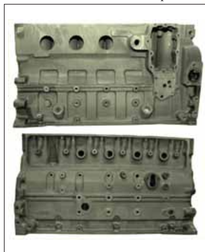
Figure 2 Second design ISB 5.9L “24 Valve” Cummins STORM block.
