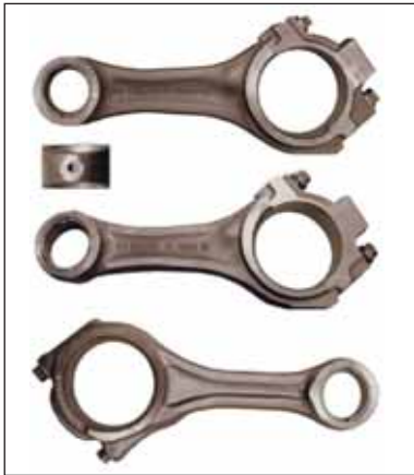
Figure 5 The first and second connecting rod designs were identical except for the oil hole in top as shown in inset. The third design rod has additional material in the forging at con rod bolt boss. All connecting rods use a tapered pin boss area.
