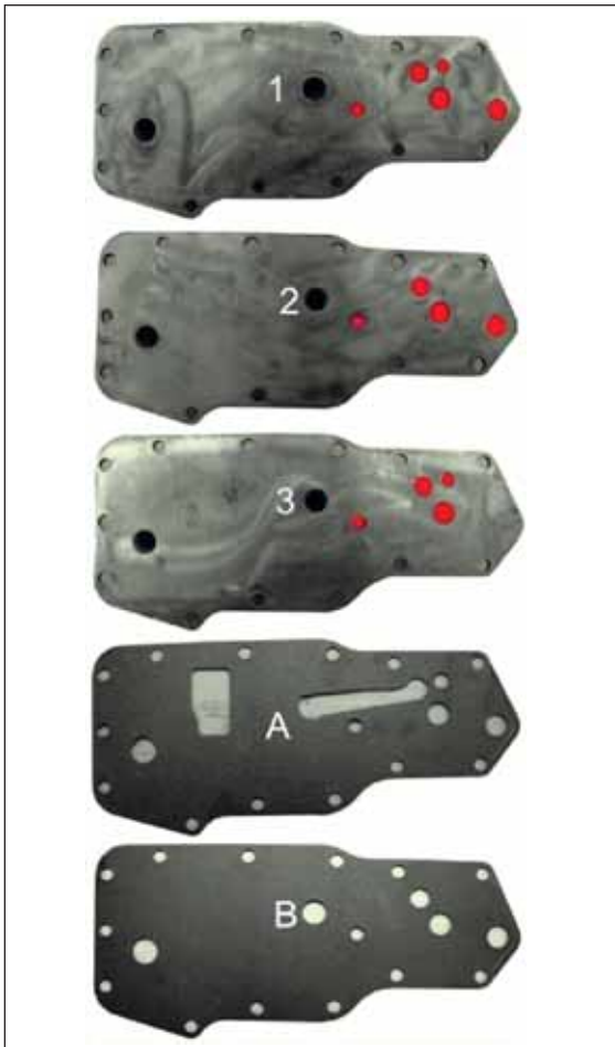
Figure 13 Oil coolers and gaskets can give you fits if used with either extremely high or low oil pressure or in the incorrect combinations
