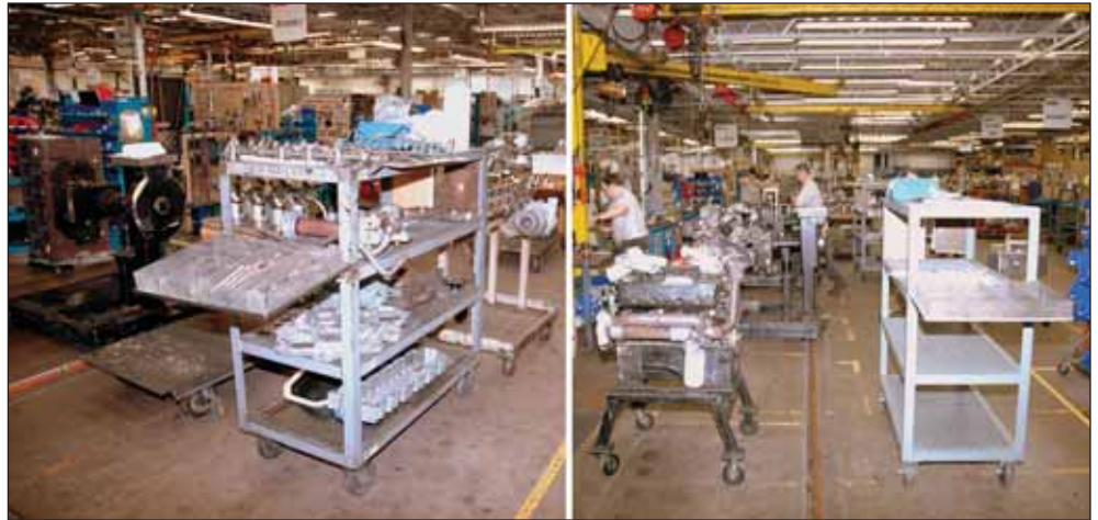
Nothing is left to chance at Reviva during assembly. On the left are all the engine sub-assemblies, right down to every bolt and nut needed. On the right is an engine on the dyno stand and an empty cart. If everything is used then nothing was left out.
