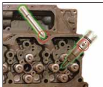
Figure 11 Attempting to remove an injector from an ISB head without first removing the fuel line adapter will permanently damage the injectors
