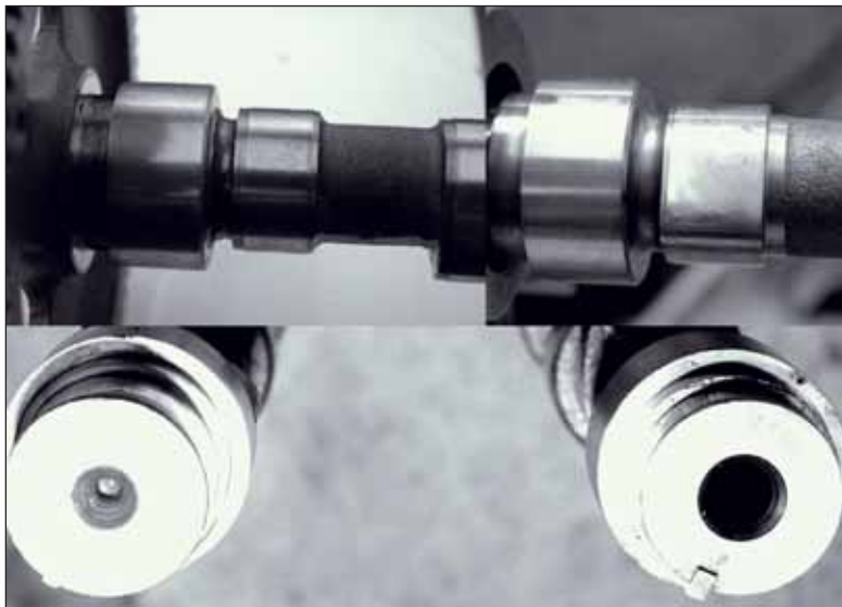
Figure 7 The first design camshaft (top left) is as cast between the first main and first lobe where the second design had a rolled radius (top right). The bottom picture explains the hole for the additional bolt for strengthening the cam bore.
