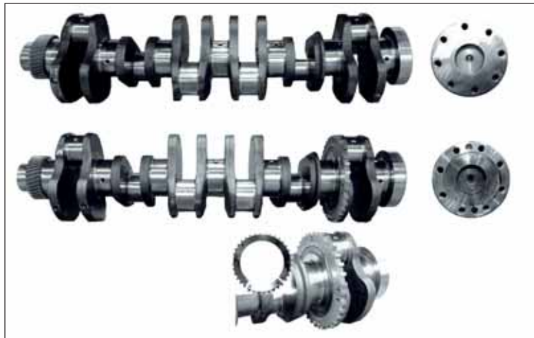
Figure 4 The upper most crankshaft is the first design used from 1983-1997.5 and from 1999.5-2002 for Dodge applications. The crank in the middle is the second design with the crankshaft position sensor trigger ring that was used from 1997.5-2002 for non-Dodge applications. The lower inlay shows the that the trigger ring is two pieces and can easily be replaced without crank removal.
